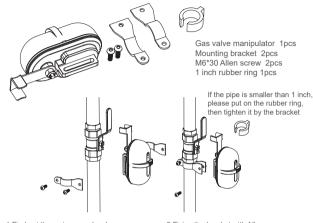
1. Find out the main gas valve, leave an adequate space for installation
